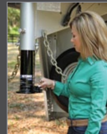
Open handle to prepare for latching
