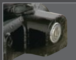
Lock is fully integrated into coupler with a mechanical shutter to keep out debris.
