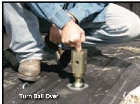
Replace Ball In Socket
